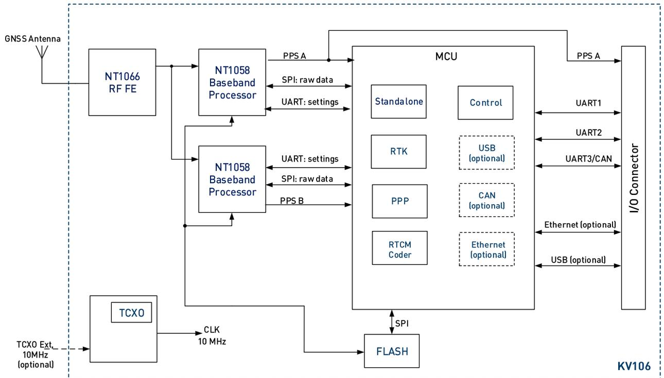
Figure 3.1– KV106 Block Diagram
