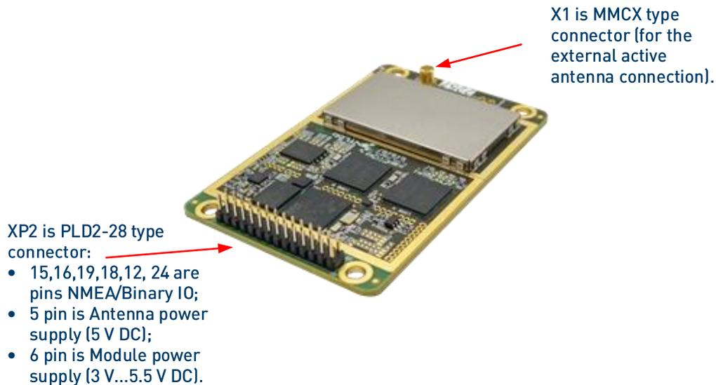
Figure 2.1– KV106 Top View<sup>1</sup>
