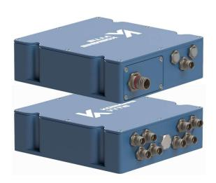
The purpose of using the KV-4AJ4.x-RO-A GNSS jamming suppressor is to ensure stable reception of the navigation signal in conditions of staged interference. The jamming suppressor should be used with the KV-AJAx phased antenna array (see the antenna array description page). The rugged A-type enclosure is designed to work at the harsh environment and to meet requirements MIL-STD 810G and MIL-STD 461G.
