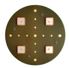
This is 4-elements Phased Array Antenna with frequency filtering at the antenna inputs and LNA on-board. Antenna Array forms the core of the system, providing exceptional signal reception and transmission capabilities.
