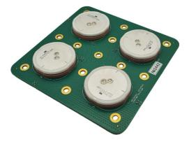
This is 4-elements Phased Array Antenna with frequency filtering at the antenna inputs and LNA on-board. The Anti-Jamming function is achieved by using it combined with Kosminis Vytis Anti-Jamming GNSS receiver which includes an Anti-Jamming GNSS processor. Signals acquired by Array Antenna are digitized and processed with KV-AJ2.x (KV-AJ2.x-OEM) high dynamic range receiver after which the navigation signals or solution is resistant to jammers.
