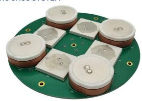
This is 4-elements Phased Array Antenna with frequency
