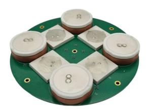
This is 4-elements Phased Array Antenna with frequency filtering at the antenna inputs and LNA on-board. The Anti-Jamming function is achieved by using it combined with Kosminis Vytis Anti-Jamming GNSS receiver which includes an Anti-Jamming GNSS processor. Signals acquired by Array Antenna are digitized and processed with KV-AJ3.3 (KV-AJ3.4) high dynamic range receiver after which the navigation signals or solution is resistant to jammers.
