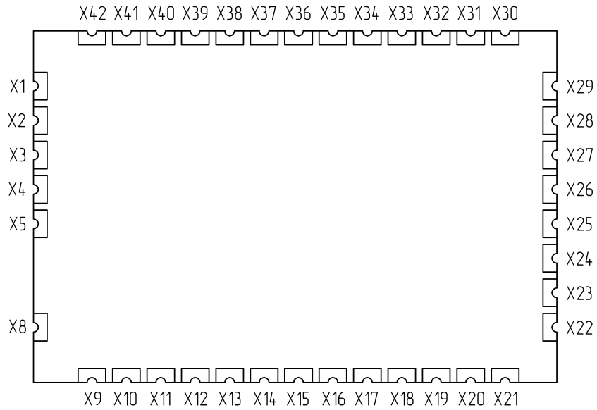
Figure 4.1 – Pinout of KV103.SMT module
