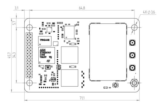
Figure 6.1- KV106 Board Layout and Dimensions
