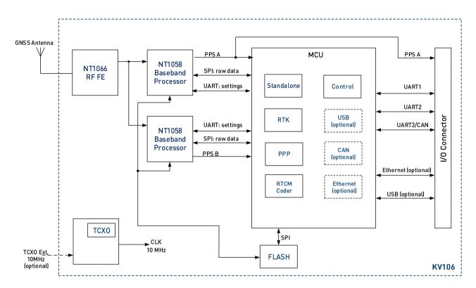
Figure 3.1- KV106 Block Diagram
